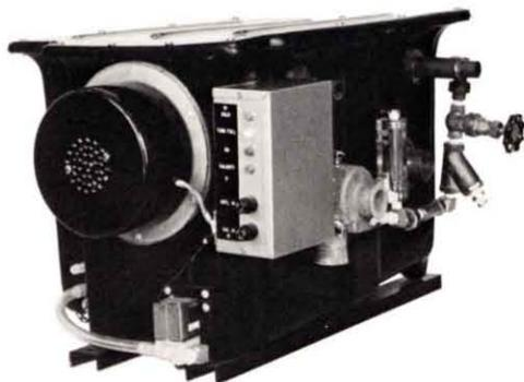
An automatic evaporator with low power drain, the model SS3 Sea-Still will make up to 100 gallons per day of drinking water. Built of Fiberglass, Monel and Cupro-Nickel, the SS3 operates on 12V DC and draws approximately 15 amps. An accessory power pack is available for use with 120-240V AC shipboard systems.
