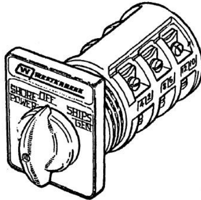
Figure 29: Shore Power Transfer Switch
