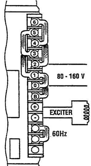
**NOTE:** IF WIRING FOR 50 HZ., THE 60 HZ. JUMPER MUST BE REMOVED FROM THE REGULATOR.
