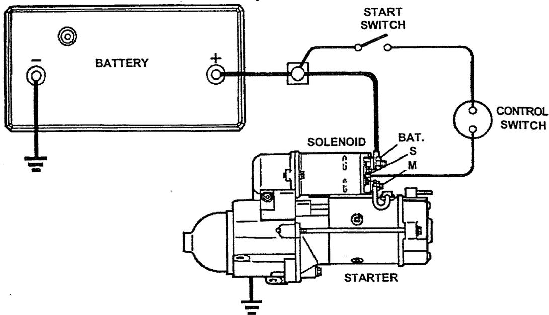
FIGURE 1. STARTER WIRING CIRCUIT
