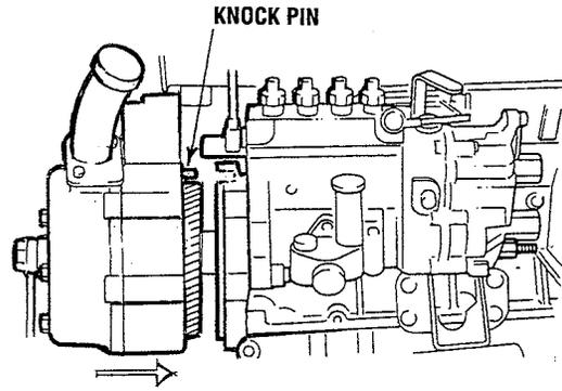
Position the injection pump so the knock pin on the timing gear case and its hole on the injection pump flange are aligned, then install the injection pump. Tighten the installation bolts to the specified torque.
