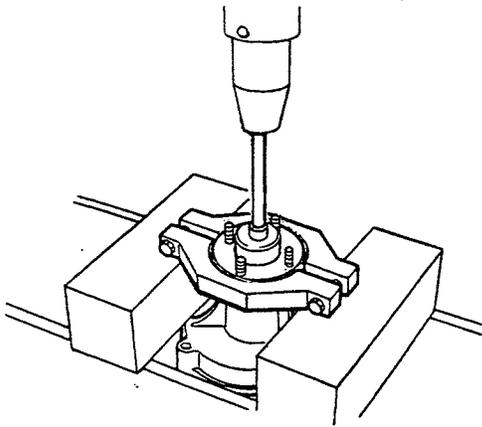
2. Press out the water pump impeller and shaft/bearing using the **water pump impeller support block** (Mazda #49 0823 146) and a press.
