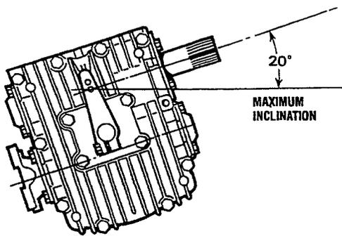
**NOTE:** When installing the gearbox, make certain that shifting is not impeded by restricted movability of the Bowden cable or rod linkage, by unsuitably positioned guide sheaves, too small a bending radius, etc. In order to mount a support for shift control cable connections, use the two threaded holes located above the shift cover on top of the gear housing. Refer to the WESTERBEKE parts list.
