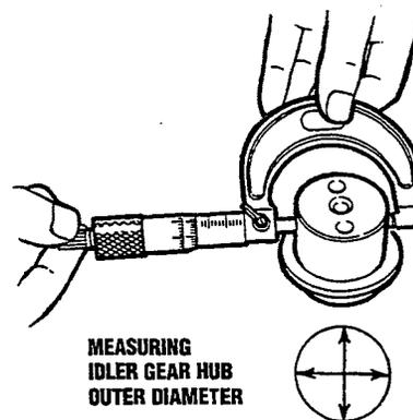
MEASURING IDLER GEAR HUB OUTER DIAMETER
