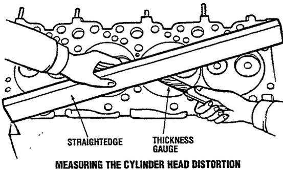
3. If the cylinder head distortion exceeds the limit, replace it.
