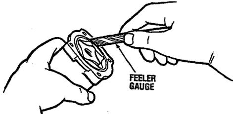
5. **Check the clearance between the rotors and the pump cover.** Inspect the end float of the rotors. Place a straightedge across the pump body and measure the clearance between the rotor and the straightedge with a feeler gauge. If the clearance exceeds the limit, replace the drive gear, drive shaft, inner rotor, outer rotor and pump body.
