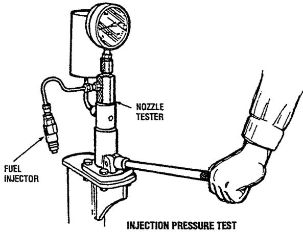
6. If the injection starting pressure is not within the specified range, adjust it by replacing the shim with one of a more appropriate thickness.
