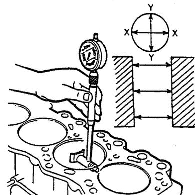
MEASURING CYLINDER LINER INNER DIAMETER
