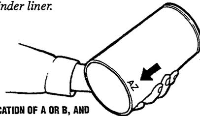
LOCATION OF A OR B, AND Y OR Z ON CYLINDER LINER
