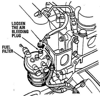
*Bleeding air from the fuel line between the engine-mounted fuel filter and the injection pump.*
