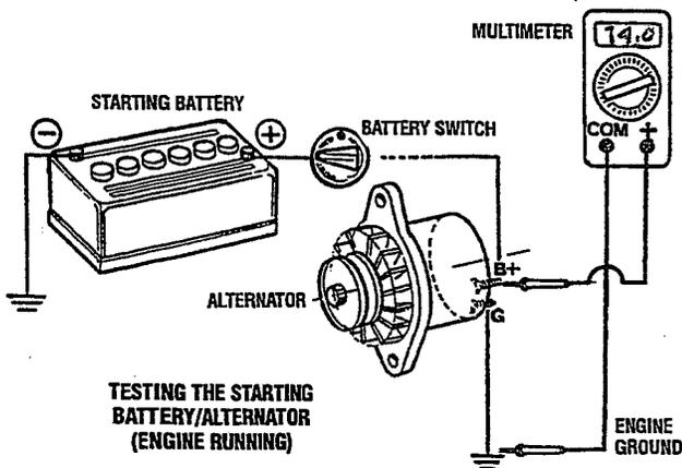
8. Start the engine again. Check the voltage between the alternator output and ground. The voltage reading for a properly operating alternator should be between 13.5 and 14.5 volts. If your alternator is over- or under-charging, have it repaired at a reliable service facility.
