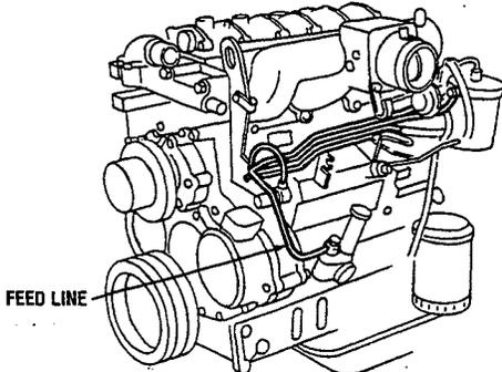
INSTALLING FUEL FEED LINE
