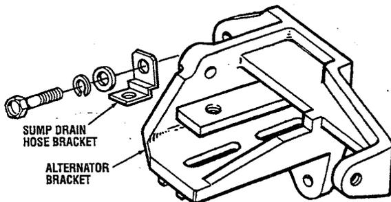
INSTALLING ALTERNATOR BRACKET
