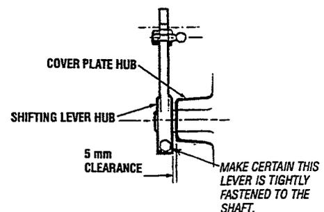
**CAUTION:** The position of the mechanism behind the actuating lever is factory-adjusted to ensure equal actuating lever travel from Neutral position N to Reverse position A and Forward position B. If this mechanism is in any way tampered with, the transmission warranty will be void.
