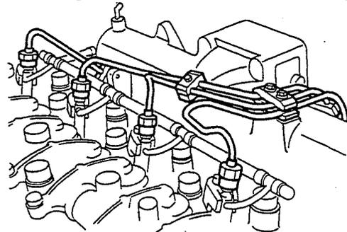
INSTALLING FUEL INJECTION LINES
