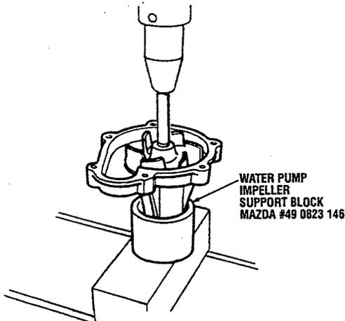
3. Tap out the seal using a pipe of the specified size.
