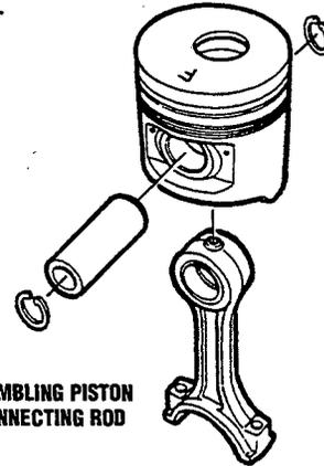
ASSEMBLING PISTON & CONNECTING ROD
