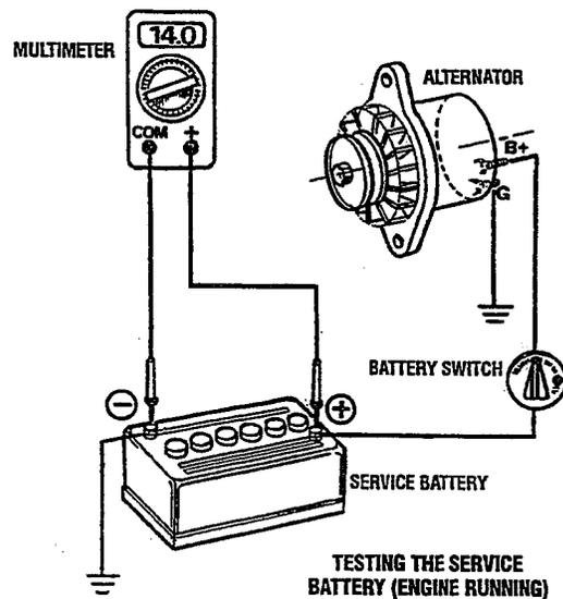
**CAUTION:** To avoid damaging the alternator diodes, do not use a high voltage tester (i.e. a megger) when performing tests on the alternator charging circuit.
