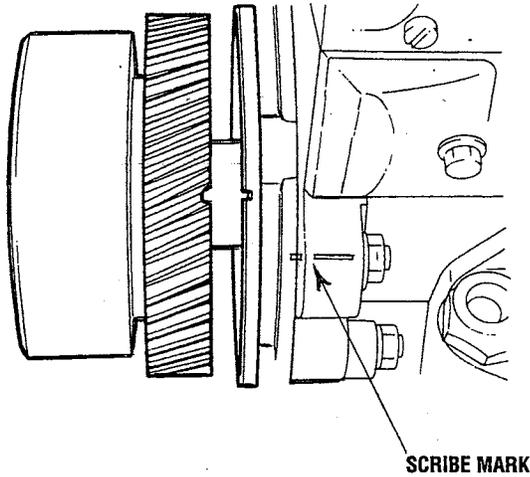
**NOTE:** When these scribe mark are properly aligned, there should be no need to check the injection timing. If, however, the injection pump or the injection pump flange has been replaced, the injection timing must be checked and, if necessary, adjusted.
