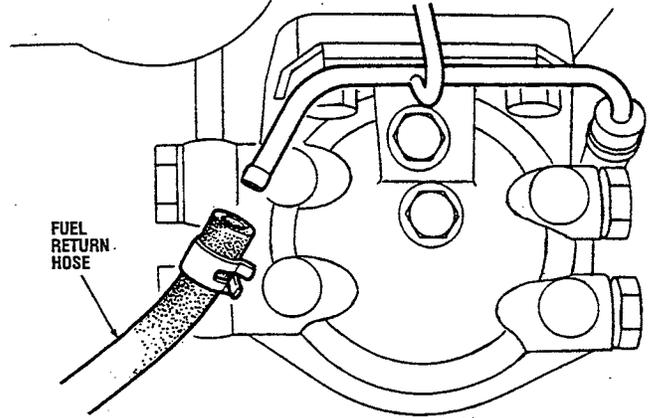
4. Repeatedly depress and release the primer until only fuel (no air bubbles) flows out of the air bleeding plug hole.
