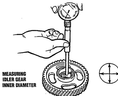
MEASURING IDLER GEAR INNER DIAMETER
