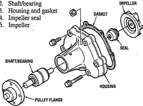
1. Press out the coolant pump pulley flange using a suitable **puller** and a press.
