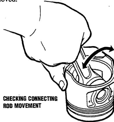
CHECKING CONNECTING ROD MOVEMENT
