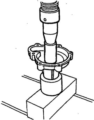
7. Press in the water pump flange using a pipe of the specified size.
