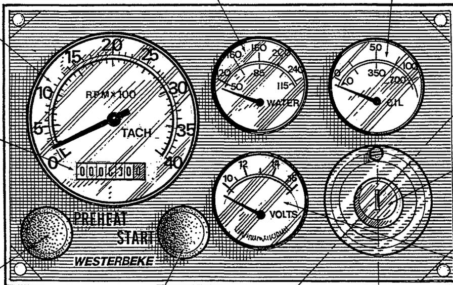
**PREHEAT BUTTON:** WHEN PRESSED, ENERGIZES THE ALTERNATOR'S EXCITER, THE FUEL LIFT PUMP, THE FUEL SOLENOID ON THE INJECTION PUMP, AND THE ENGINE'S AIR INTAKE HEATER. IT BYPASSES THE ENGINE'S OIL PRESSURE ALARM SWITCH. IN ADDITION, THIS BUTTON ENERGIZES THE START BUTTON.
