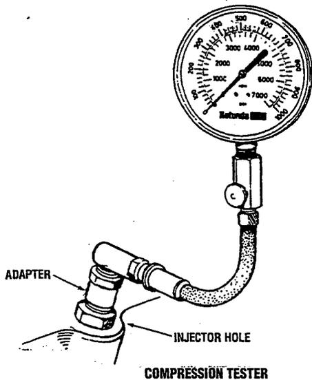
If a weak cylinder is flanked by healthy cylinders, the problem is either valve- or piston-related. Check the valve clearances for the weak cylinder, adjust as needed, and test again. If the cylinder is still low, apply a small amount of oil into the cylinder to seal the rings, and repeat the test. If the compression comes up, the rings are faulty.
