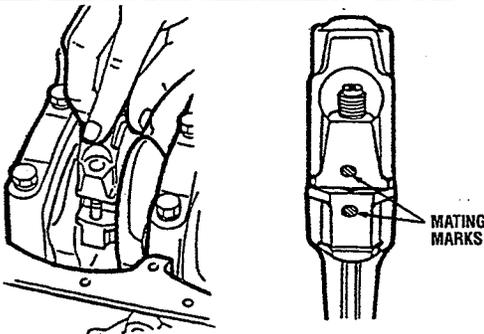
INSTALLING CONNECTING ROD BEARING CAP
