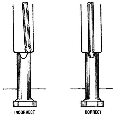
INSERTING PUSH RODS
