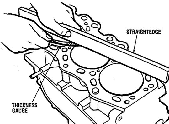
MEASURING CYLINDER BLOCK DISTORTION
