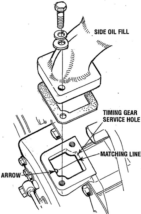
Remove the gear case side oil filter neck. This will expose the gear cover service hole.
