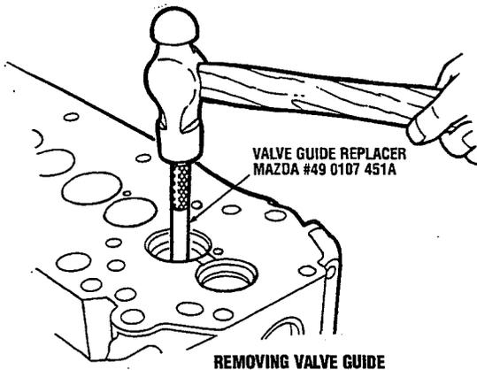
REMOVING VALVE GUIDE
