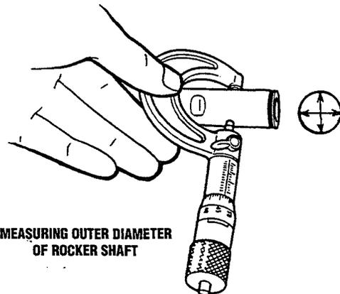
MEASURING OUTER DIAMETER OF ROCKER SHAFT
