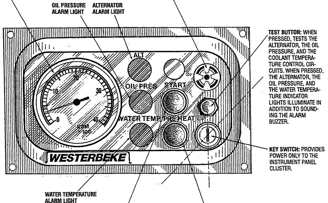
**TEST BUTTON:** WHEN PRESSED, TESTS THE ALTERNATOR, THE OIL PRESSURE, AND THE COOLANT TEMPERATURE CONTROL CIRCUITS. WHEN PRESSED, THE ALTERNATOR, THE OIL PRESSURE, AND THE WATER TEMPERATURE INDICATOR LIGHTS ILLUMINATE IN ADDITION TO SOUNDING THE ALARM BUZZER.
